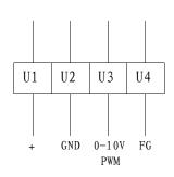
The fan provides a speed output signal, output signal drawing see under annex. Vfg and pull up resistor are connected by customer. Vfg= (3-30) VDC, R  $\geq$  1000  $\times$  (Vfg)  $\Omega$
